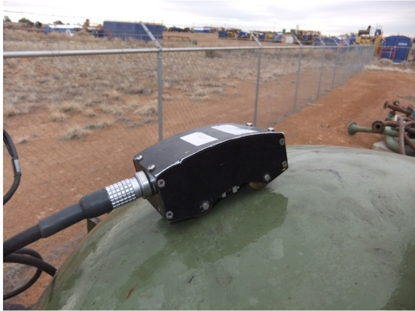
Figure 26 "Pocket-UT" transducer assembly shown on a vessel top head, courtesy of Sandstone Engineering.
