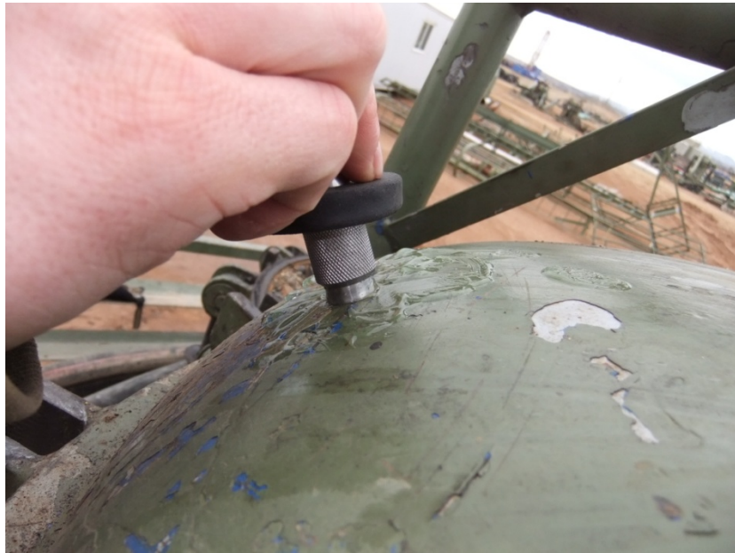
Figure 32 Topcoat ultrasonic transducer and couplant on pressure vessel head
