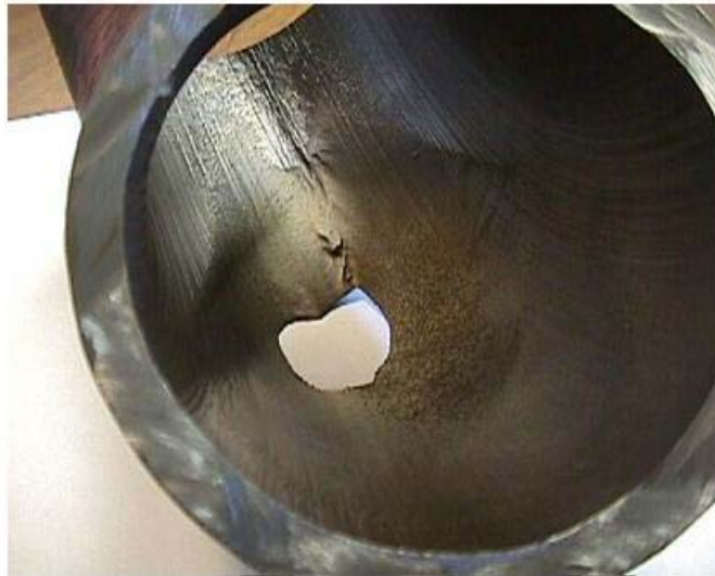
Figure 4 Erosion of return bend [8].
