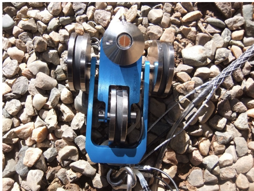
Figure 29 Bottom view of manual UT crawler and spring loaded transducer
