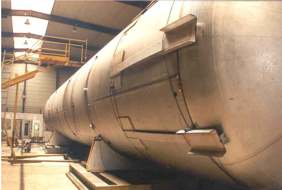
Figure 40 Acoustic emission monitoring of pressure vessel final testing [17].
