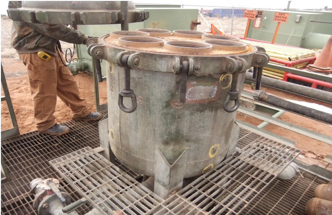
Figure 20 Filter Specialists, Inc. sock filter vessel on portable skid with quick opening closure opened.
