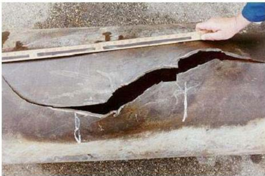
Figure 1 Brittle fracture failure during hydrotest of 20-inch OD carbon steel pipeline [8].
