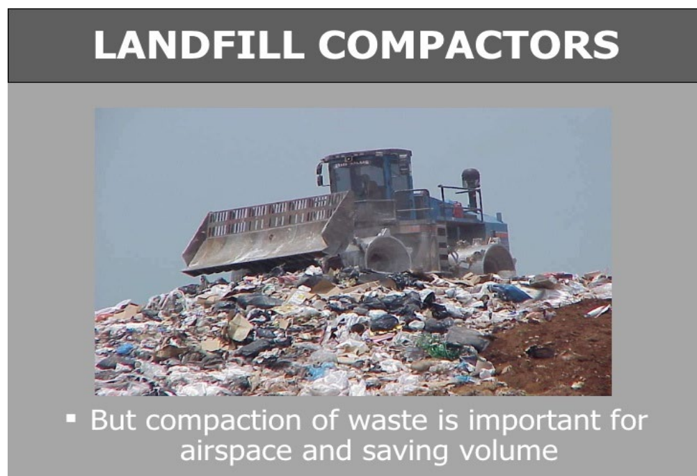
Figure 11: Landfill Compactor being used in working face
